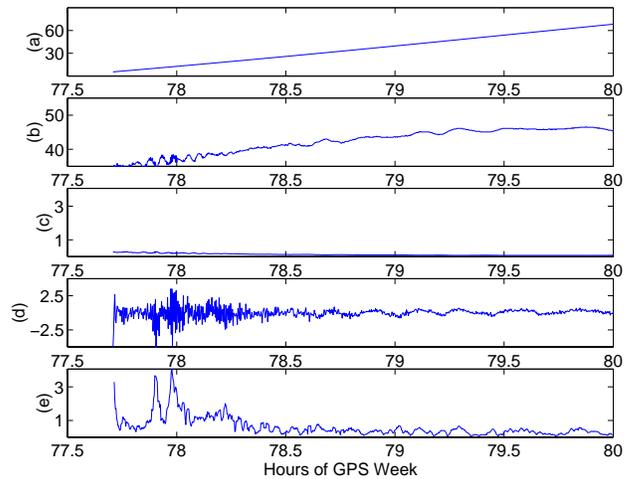
Figure 3: Weighting functions comparison using synthesized P-code observations collected from SV22. (a) SV elevation (deg.). (b) Signal  $C/N_0$  (dB-Hz). (c) Pseudorange precision (m). (d) Pseudo-multipath (m). (e) Pseudo-multipath precision (m)
