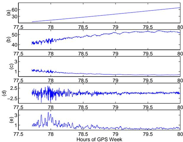
Figure 2: Weighting functions comparison using C/A-code observations collected from space vehicle (SV) 22. (a) SV elevation (deg.). (b) Signal  $C/N_0$  (dB-Hz). (c) Pseudorange precision (m). (d) Pseudo-multipath (m). (e) Pseudo-multipath precision (m).
