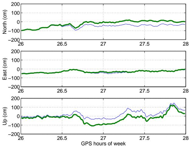
Figure 10: Un-weighted (thin blue line) and de-weighted (thick green line) pseudorange and carrier-phase forward-filter point positioning component errors for Algonquin data set.
