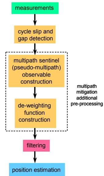
Figure 1: Measurement processing flow augmented by multipath mitigation modules.
