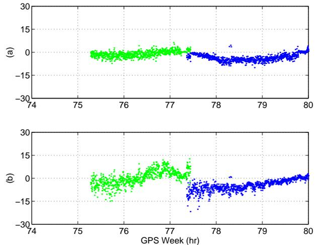
Figure 8: Pseudorange residuals (in metres) for SV11 (light green) and SV06 (dark blue) from un-weighted solution (a) and de-weighted solution (b) for Ganong Hall data set.
