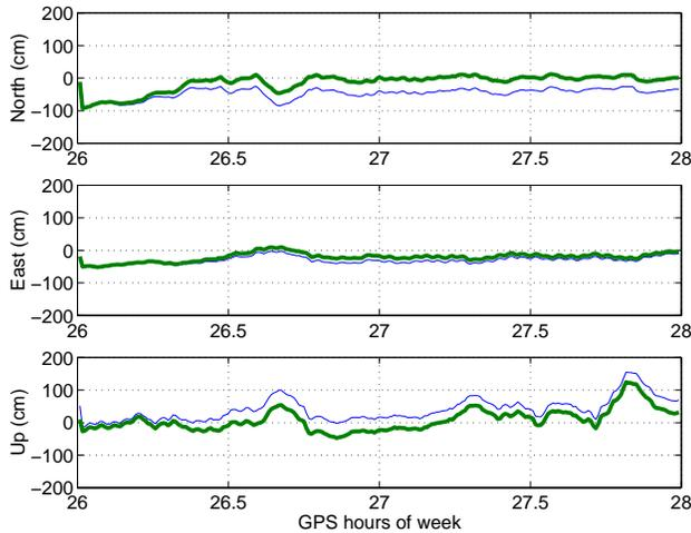
Figure 12: Un-weighted (thin blue line) and de-weighted (thick green line) pseudorange and carrier-phase smoothed point positioning component errors for Algonquin data set.
