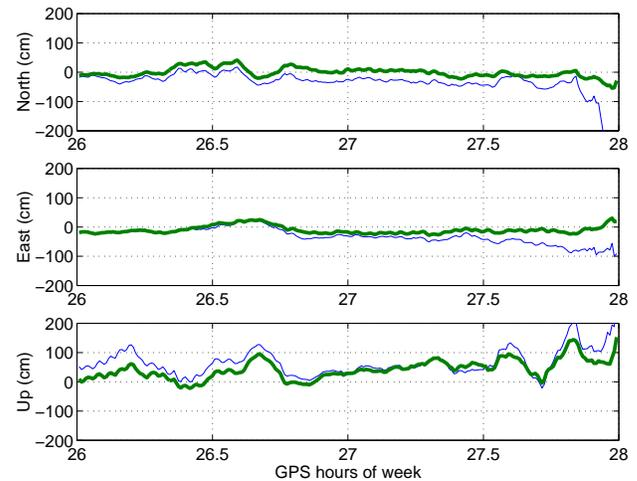
Figure 11: Un-weighted (thin blue line) and de-weighted (thick green line) pseudorange and carrier-phase backward-filter point positioning component errors for Algonquin data set.
