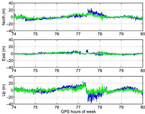
Figure 7: Un-weighted (dark blue) and de-weighted (light green) pseudorange point positioning component differences from the mean for Ganong Hall data set.
