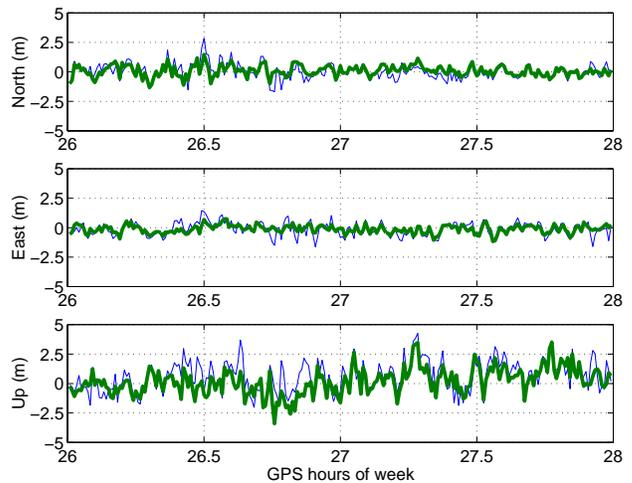
Figure 9: Un-weighted (thin blue line) and de-weighted (thick green line) pseudorange point positioning component errors for Algonquin data set.
