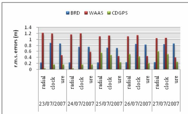
Figure 4. r.m.s. errors for the radial orbit component, clock and URE from July 23, 2007 to July 27, 2007.
