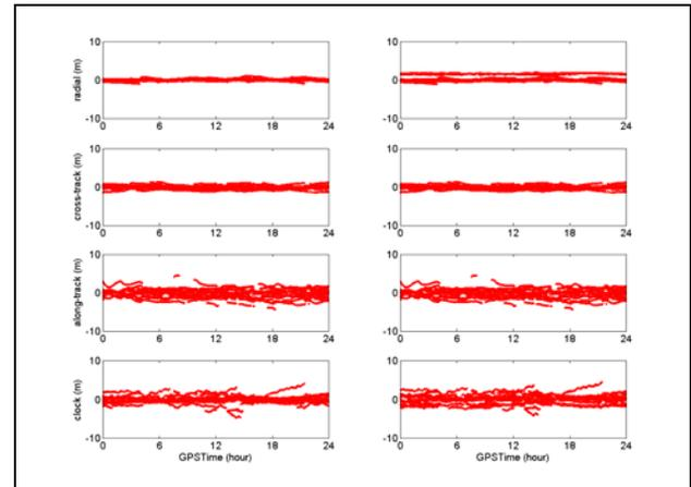
Figure 1. Broadcast orbit and clock errors on July 23, 2007. The left panel shows the broadcast orbit and clock errors computed by using the NGA offsets and the right panel shows those errors computed by using the IGS offsets.
