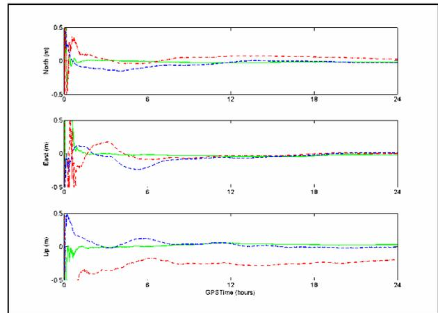
Figure 5. Precise point positioning results (static case) with IGS products (green), CDGPS corrections (blue) and WAAS corrections (red) at station ALGO on July 23, 2007.
