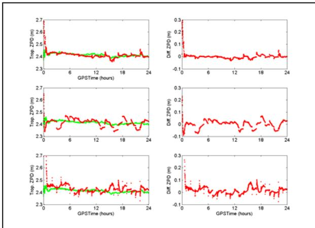
Figure 6. Estimated tropospheric delays with the different orbit and clock products at station ALGO on July 23, 2007. The top panel shows the results with the IGS products, the middle panel shows the results with the CDGPS corrections and the bottom panel shows the results with the WAAS corrections. The green colors show the troposphere delays from the NRCan PPP software.
