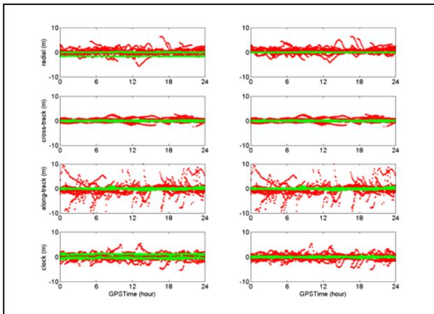
Figure 2. CDGPS- (green) and WAAS- (red) corrected orbit and clock errors on July 23, 2007.
