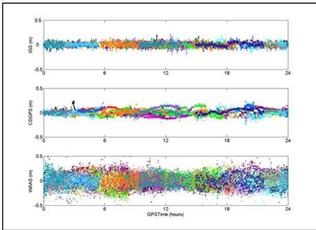
Figure 7. Residual errors for the PPP results at station ALGO on July 23, 2007. The scale of the WAAS residuals were fixed to  $\pm 0.5$  m to see the detailed view.
