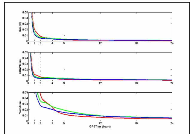
Figure 8. Convergence of the sigma with the different satellite orbit and clock corrections. The red color shows the sigma for the north component and the green color represents the east component. Finally the blue color shows the up component of the sigma in time.
