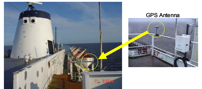
Figure 13. Onboard GPS antenna under multipath rich environment.
