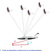
$\boldsymbol{g}^*$  Total acceleration measured by accelerometers. Total acceleration is composed of:  $\boldsymbol{g}$  - the earth's gravity field and  $\boldsymbol{a}$  - acceleration due to the motion of the aircraft derived at a point in the aircraft from GPS position estimates
