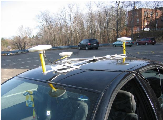
**Figure 5:** Kinematic test setup (there is a huge blockage – the façade of a building with several floors - not visible in the picture, and serving as the effective reflector in the tests, because of its dimensions and smoothness of its surfaces).
