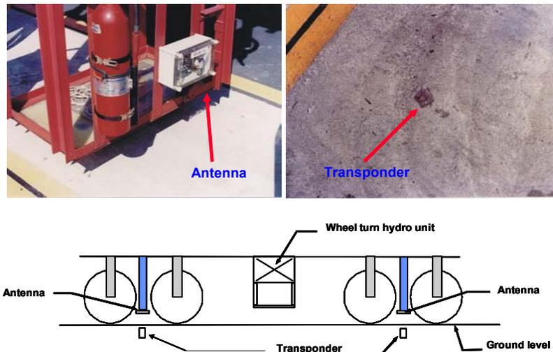
Figure 5: RTGC auto-steering system based on the transponder technology.
