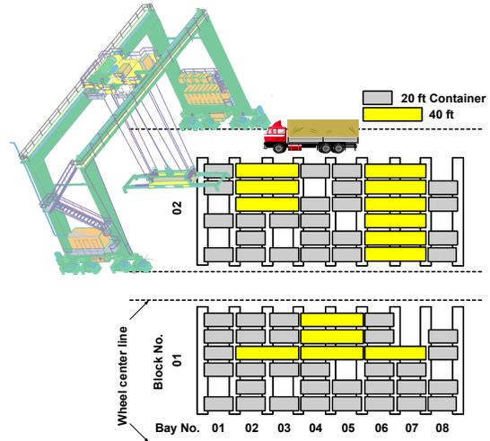
Figure 1: (left) RTGCs handling containers at Kwangyang Port and (right) sketch of a container yard.
