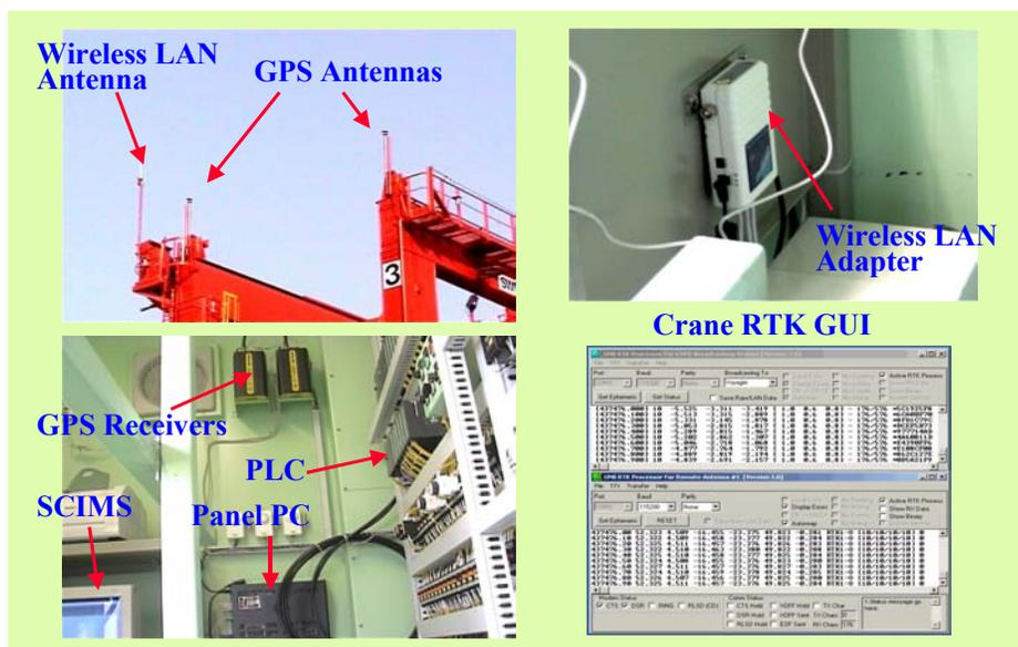
Figure 10: System components at the crane station.
