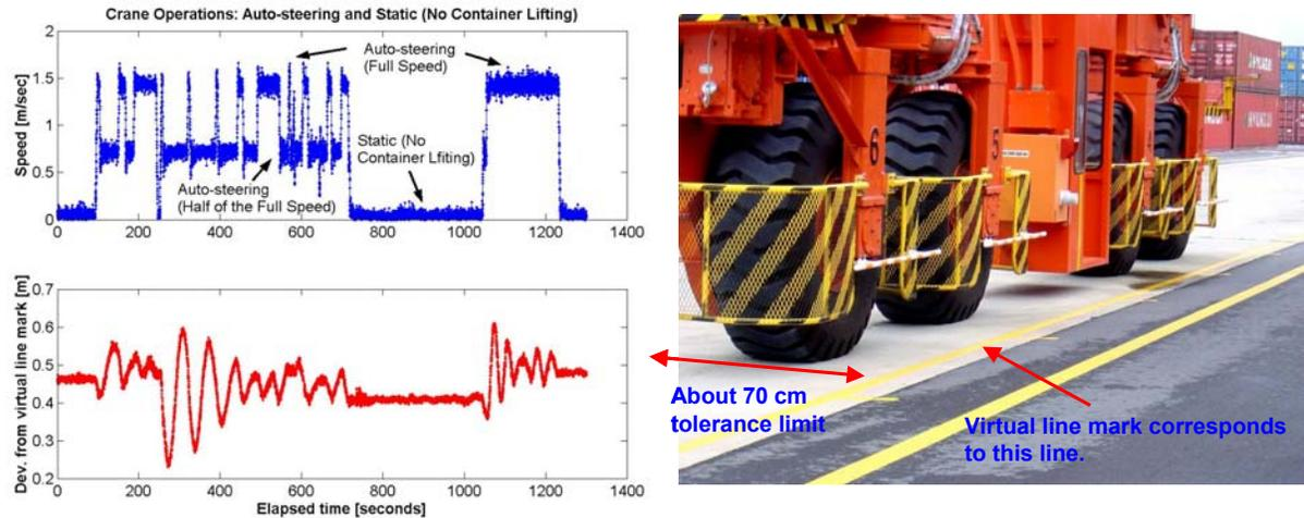
Figure 12: (left) Crane dynamics (speed and deviation) during the test run of the bottom panel in Figure 11(right) and (right) an RTGC's front and rear wheels moving along the concrete lane (corresponding to a virtual strip with an order of 70 centimetres in width and 500 metres in length).
