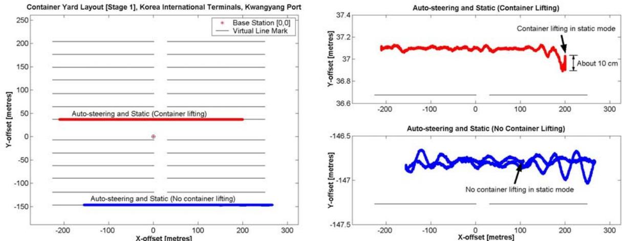
Figure 11: (left) Tracks of RTGC test runs (overlapped on the container yard layout) and (right) magnified tracks of the test runs. The sinusoidal pattern of wheel deviation is typical in auto-steering mode. The effects of lifting a container are oscillations along the Y-offset axis (top panel in Figure 11(right)).
