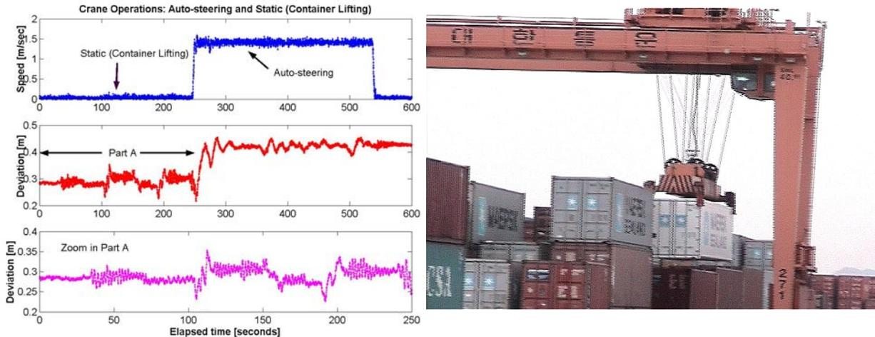
Figure 14: An RTGC introducing high dynamics to the GPS antennas on lifting a container.
