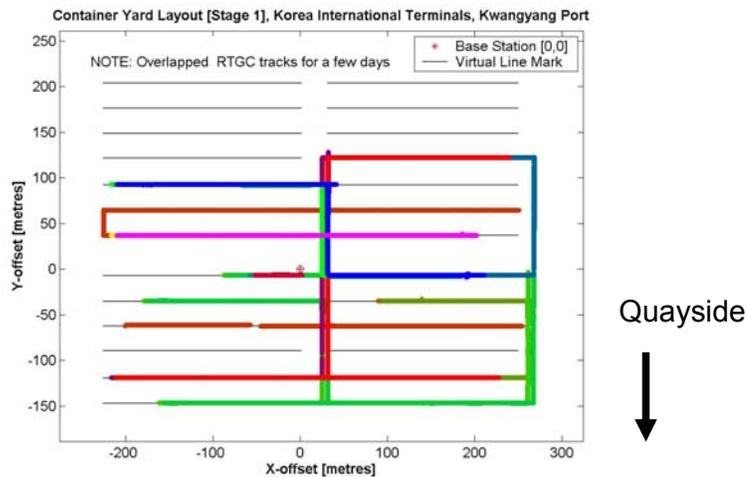
Figure 7: Example of an electronic map with virtual line marks. The tracks of RTGCs during auto-steering test runs are overlapped on the map.
