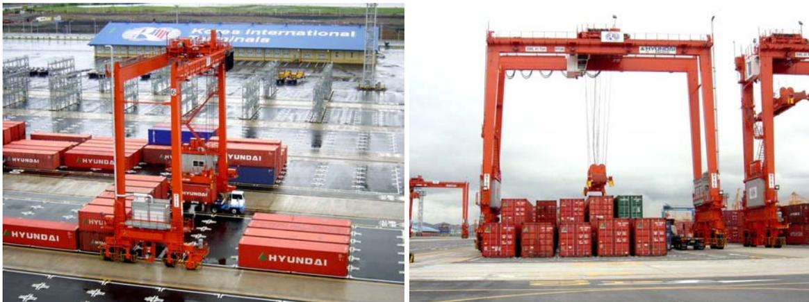
*Figure 3: RTGCs in operation: (left) lifting a container off a truck platform and (right) lowering a container into a desired location.*
