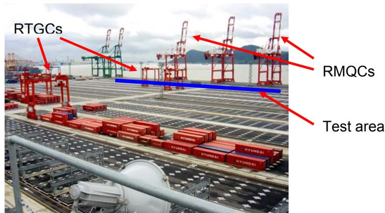
Figure 13: Auto-steering test under multipath-rich environment and transient signal-interruption due to obstacles (especially, RMQCs) in the vicinity of an RTGC.
