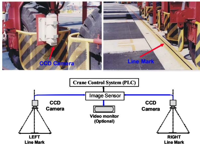
Figure 6: RTGC auto-steering system based on the CCD camera image processing technology.
