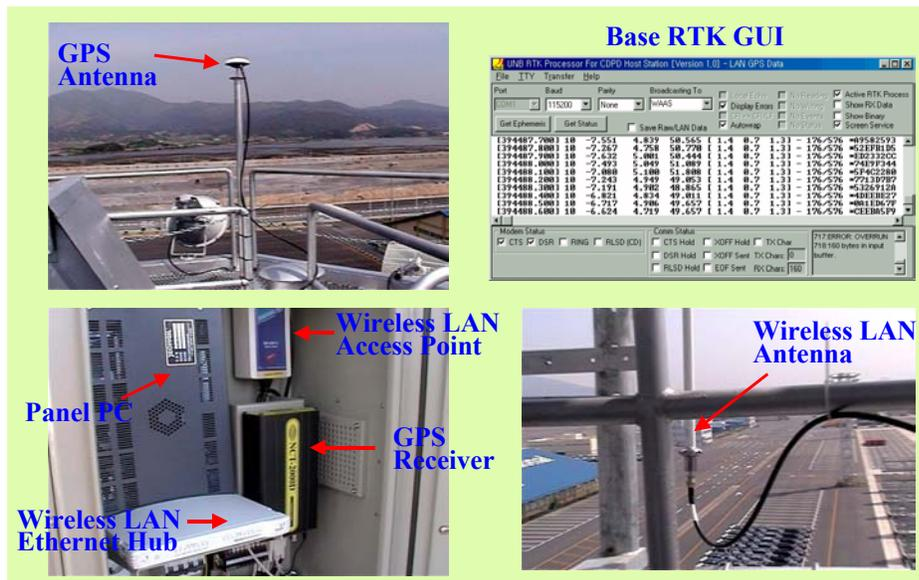
Figure 9: System components at the base station.
