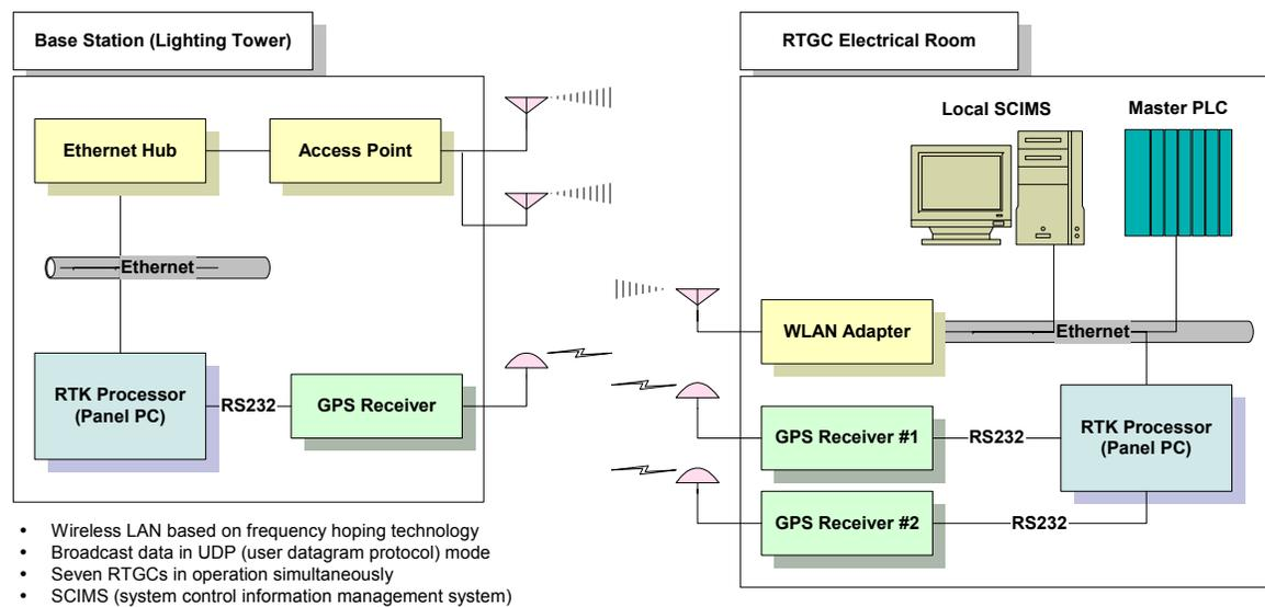
Figure 8: Sketch of the RTGC auto-steering system based on GPS RTK technology.
