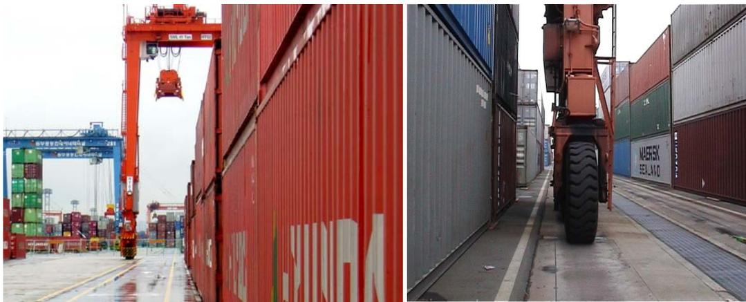
*Figure 4: RTGCs driving over long distances completely straight in quite narrow spaces.*
