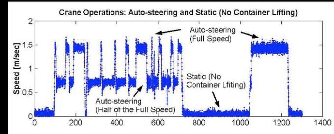
To enable control in automatic mode, UNB has developed an ultrahigh-performance GPS RTK software for gantry crane auto-steering. The UNB RTK system determines the position and orientation of the crane every one tenth of a second with accuracy better than 2 centimetres with extremely high reliability.
