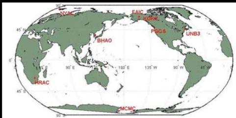
IGS has organized a network of L2C capable GPS receivers which have been established in different places. One of these stations is UNB3, operated by UNB. The role of this project is to analyze the quality of the new signal, as well as the impact of its use for positioning and navigation.
