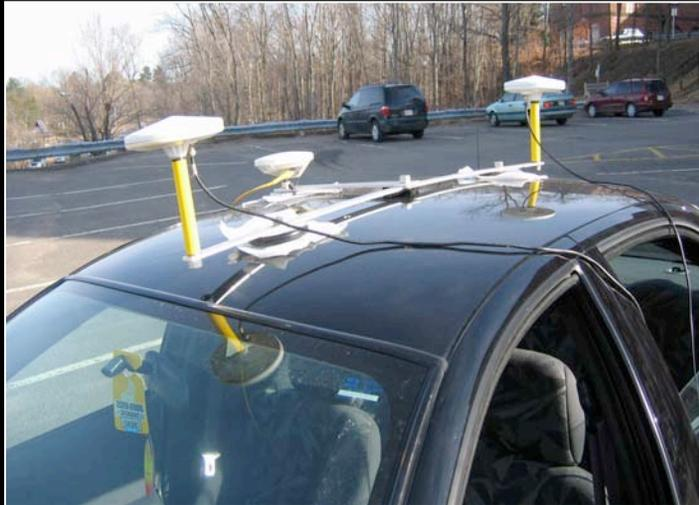
Phase multipath is probably the most difficult error to model in real-time, cm-level GNSS applications. At UNB, we have been designing strategies to tackle this effect using multipath-physical models, and precise platform dynamics/attitude. They are suitable for applications such as RTK vehicle navigation, machine guidance, attitude systems, etc.
